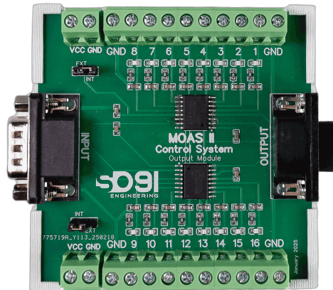
16-output module — INPUT (left) and OUTPUT (right) DB9 chain ports; VCC/GND and INT/EXT jumper visible at each end of both terminal rows
