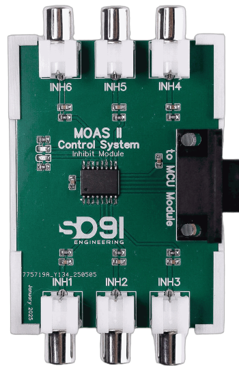
Inhibit module — six configurable RCA outputs (INH1–INH6) and a single DB9 port to the MCU module
