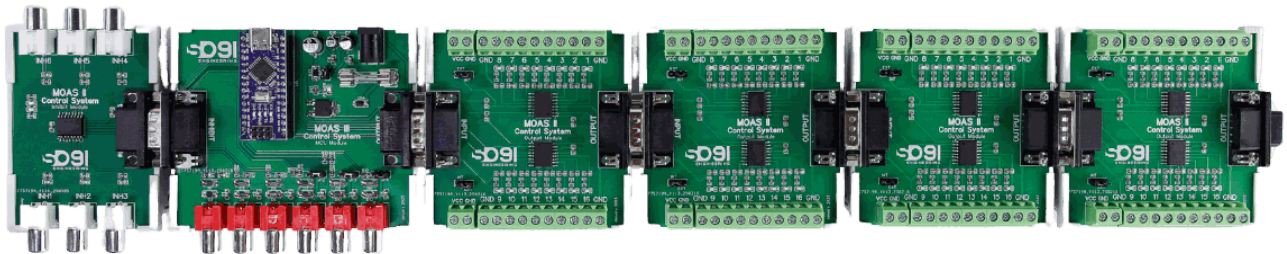
A typical set: Inhibit module — MCU module — four 16-output modules, chained left to right
